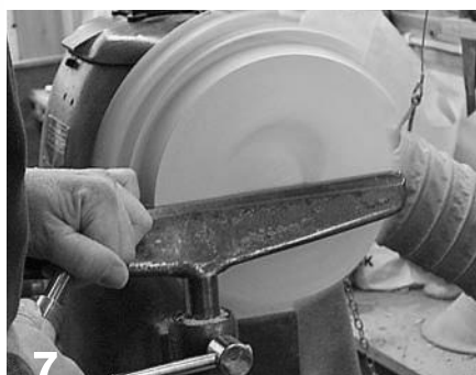
7 Cut away the bulk of the off-center rim. Work from the outside in stages, pivoting the gouge into the blurred spinning wood.
