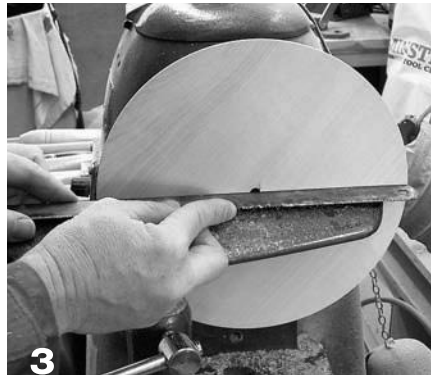
3 Turn a flat top to the platter and check with a straightedge.
