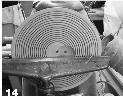
13 Start to hollow out the platter, which is mounted on the newly cut recess.
