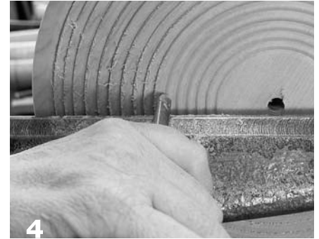
4 With a \frac{3}{8} " spindle gouge, add a series of beads to the platter.
