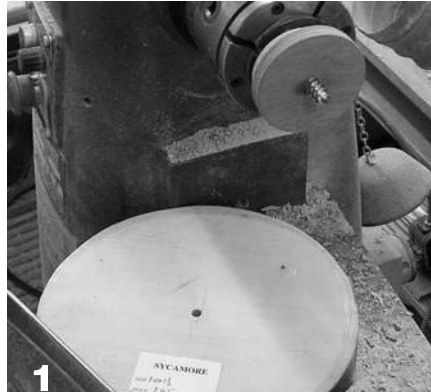
1 Start with a sound blank, roughly 10" in diameter and \frac{1}{2} " to 2" thick. Mount the stock on a screw chuck like normal.
