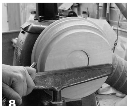
8 With the lathe stopped, it is easy to see how the offset mounting affects the cutting of the platter's rim.
